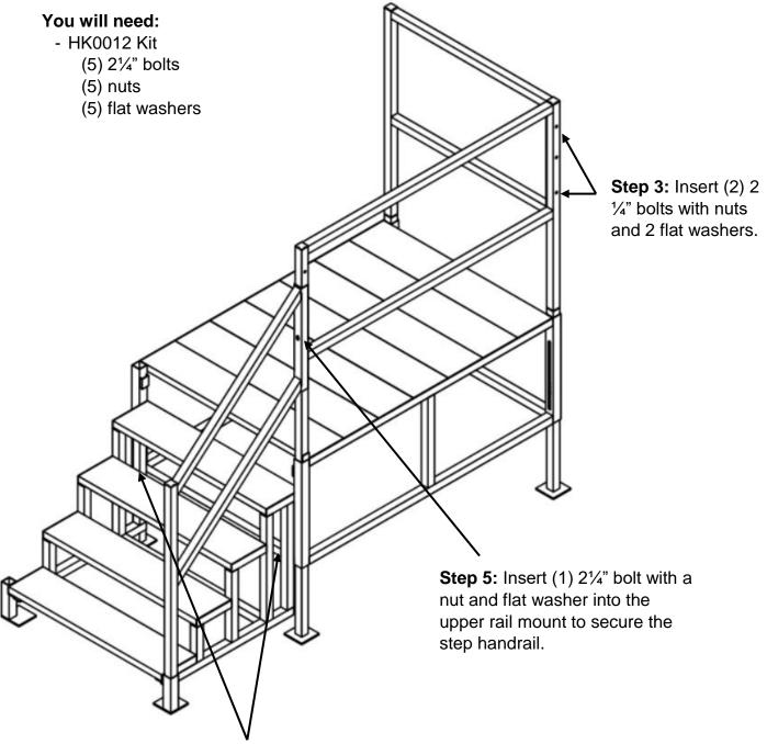
**Step 4:** Insert (1) 2 ¼" bolt with a nut and flat washer on either side of the steps through the mounting bracket on the back side of the step riser.
