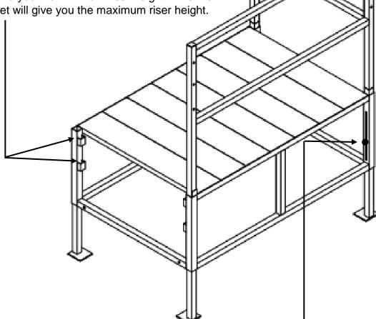
**Step 1:** Insert the platform leg, adjust it for the desired height, and insert (1) 1" bolt with 1 flat washer and 1 split lock washer. Then tighten the bolt. Repeat for the remaining platform legs.
